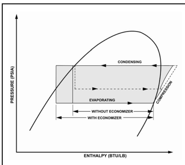
Liquid refrigerant enters the flooded evaporator uniformly where it absorbs heat from water flowing through the evaporator tubes, and vaporized. The vaporized refrigerant is drawn into the compressor suction port where the positive displacement compression begins.
