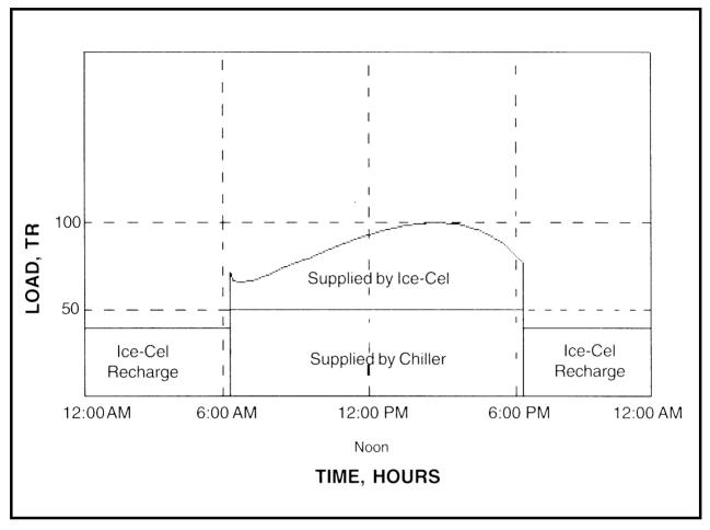
**With Partial Storage,** the liquid chiller is used at night to recharge the Ice-Cel and during the day to supplement the Ice-Cel in serving the air conditioning load. Using the same building example as above, we might choose to use 2 Ice-Cels, with 480 TR-hours storage capacity.
